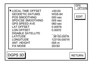
Figure 11-8 GPS SETUP options menu
